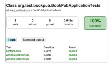
8. The more curious minds can also click on the **Standard output** button in order to see the runtime application logs that are produced during the execution of the test.
